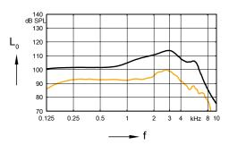
Max. Output sound pressure level  $(L_1 = 90 dB)$
